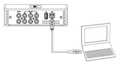
Connect a PC to Computer connection terminal of M4 with the included USB cable.
